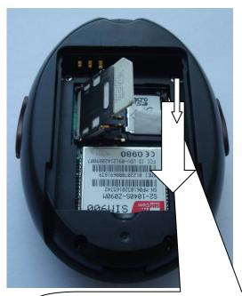
Fasten downwards ,make sure the SD card is mounted
