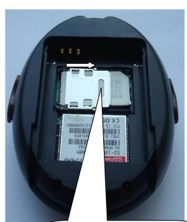
SD card is mounted, then fasten the sim card rightwards
